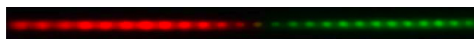
FIG. 2 Observed fringe pattern. Fringe contrast and spacing vary with the wavelength. The reduced brightness between red and green is due to the colour characteristic of the CCD camera. Here, d=100\ \mu\text{m} and p=20\ \mu\text{m} .
