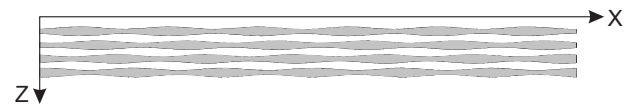
FIG. 2 Cross-section of a model paper sample used in the Monte Carlo simulation of OCT images. The sample comprises 5 fibril layers and 4 air layers. The size of the presented cross-section is 1000 by 140 \mu\text{m} . A-scans are performed consecutively along the z -axis at different x values.
