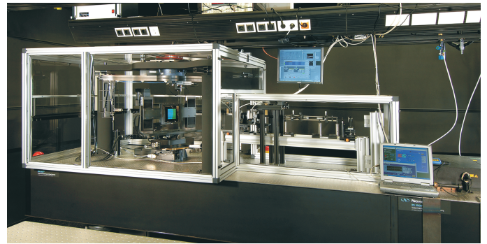
FIG. 3 Photo of the DUV hybrid scatterometer. The enclosure can be flushed with nitrogen to avoid absorption by \text{O}_2 and \text{O}_3 .
