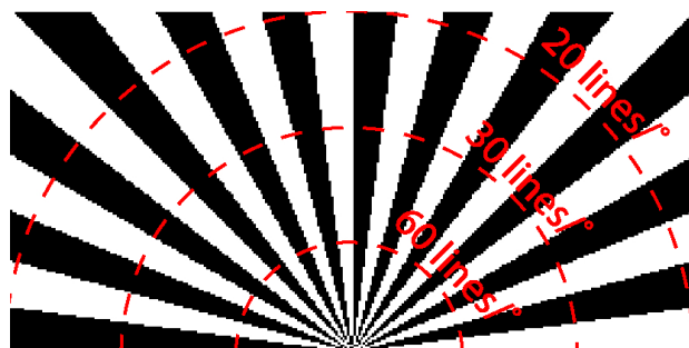
FIG. 5 Ideal image of the Siemens star obtained in a central fragment of the imaging plane with dimensions 0,30 mm × 0,15 mm.
