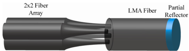
FIG. 1 Phase-locking fiber laser design showing the TMFD end section. A 2 \times 2 fiber amplifier array is coupled into a 2 \times 2 set of SM fibers which are fused onto a LMA fiber in a regular rectangular geometry. A partial reflector acts as the output coupler is fabricated on the opposite end of the LMA fiber. Also, there could be fiber Bragg gratings which 100% pass the pump and 100% reflect the signal at the input end of each fiber amplifier to form the laser cavity.
