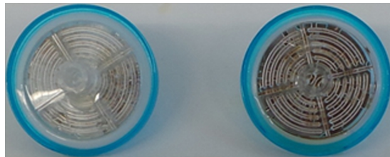
FIG. 4 Two examples (FU12 and FU18) show minimal residue after a last filtration of the solutions over 2 µm pore size filters.
