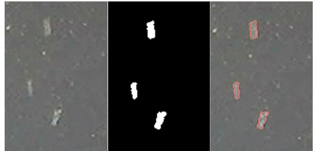
FIG. 4 (left) 100x160 pixel section of an original image. (middle) Binary image after optical flow analysis. (right) Superimposed outlined edges in the original image for illustration of object detection.
