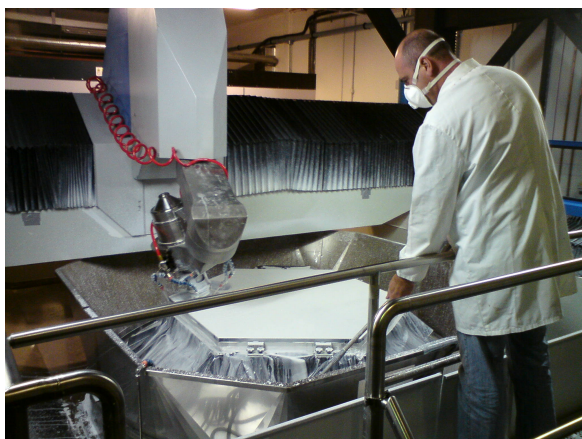
FIG. 1 Segment polishing on Zeeko IRP1600 machine at the National Facility.
